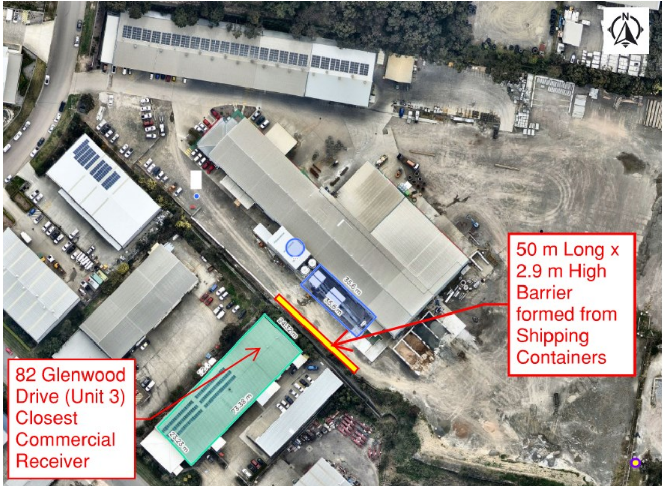
Figure 8.1 Proposed Barrier Location at South-West Site Boundary
