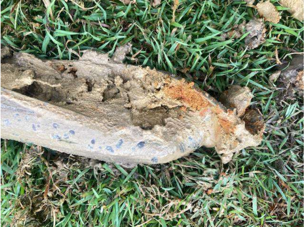
Photograph 5 – Residual clay with weathered rock inclusions
