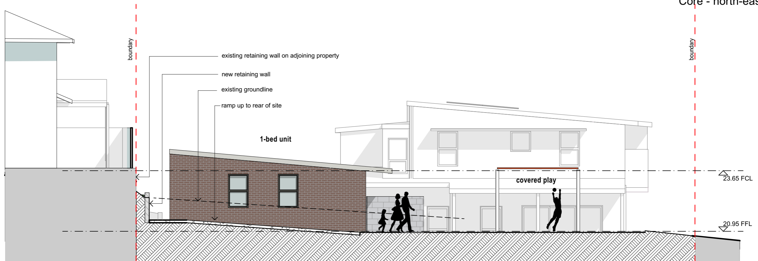
accessible unit - north-east elevation
