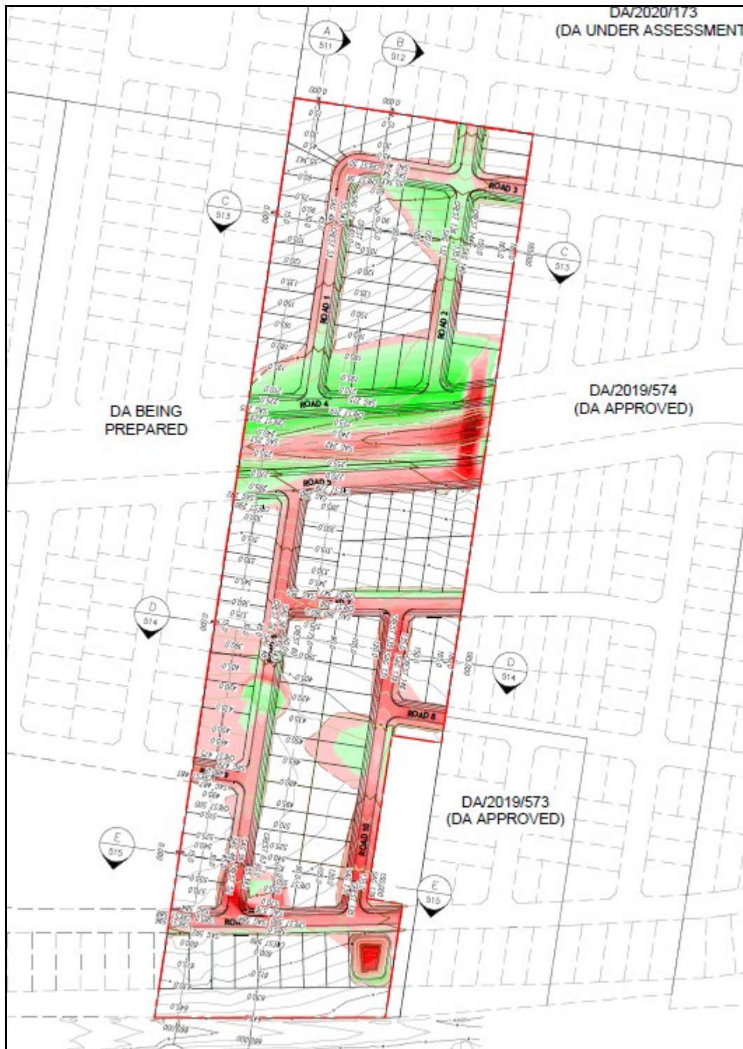
Figure 17: Earthworks Plan (Source: ADWJ, 2023)
