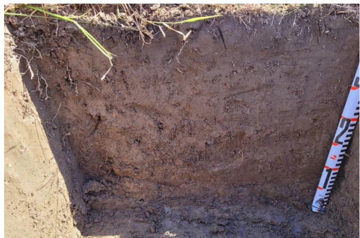
Plate 53: Photo of typical soil profile as observed in TP 2 Northern Wall
