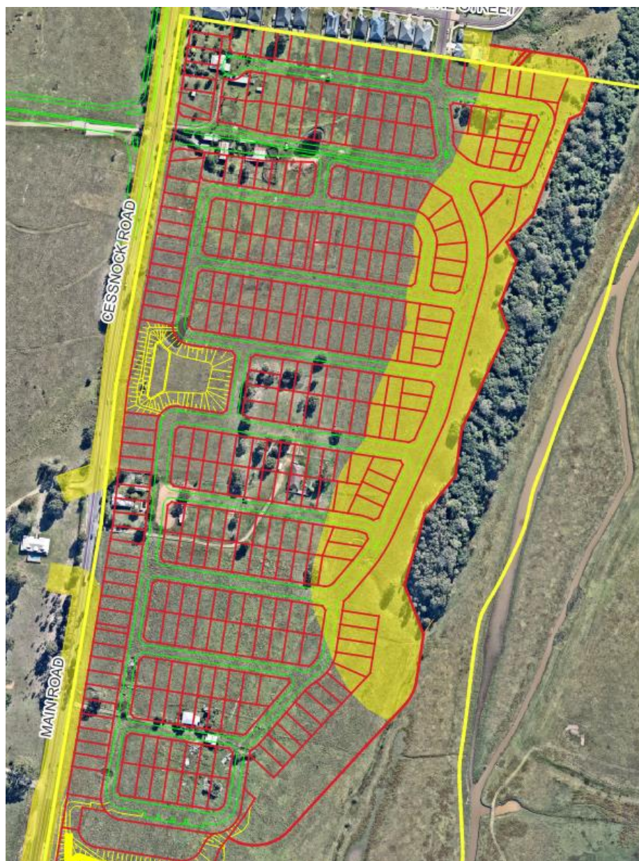
Figure 12: Subdivision Plan overlaid with 100 metre buffer from bushfire hazard and 30 metre buffer from grassland hazard
