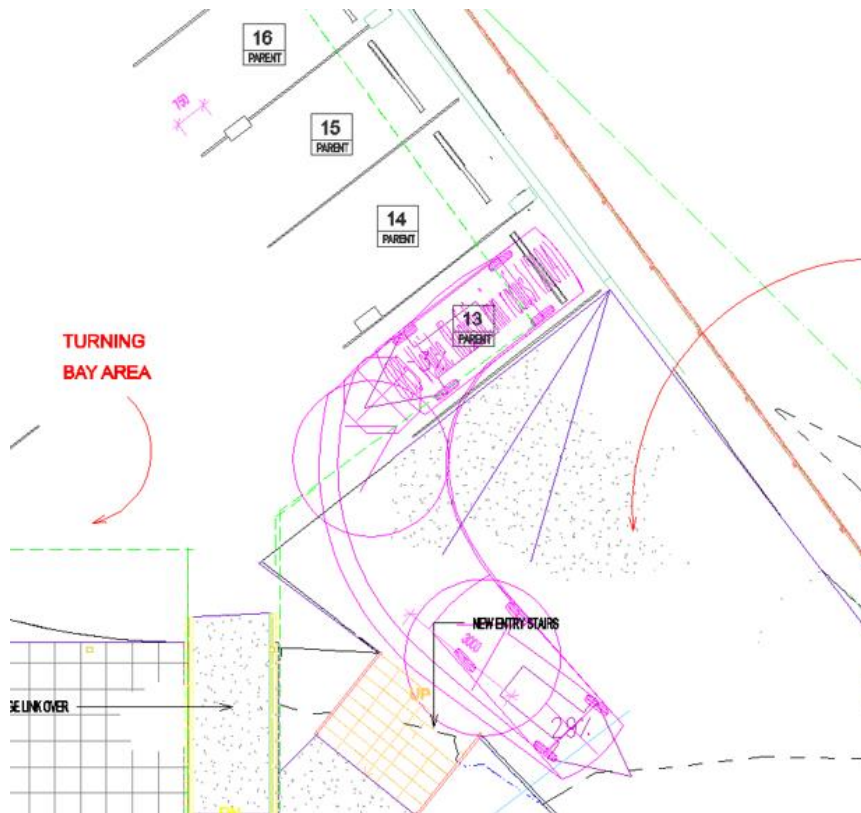
Figure 6-4: Parking Space '13' Forward OUT
