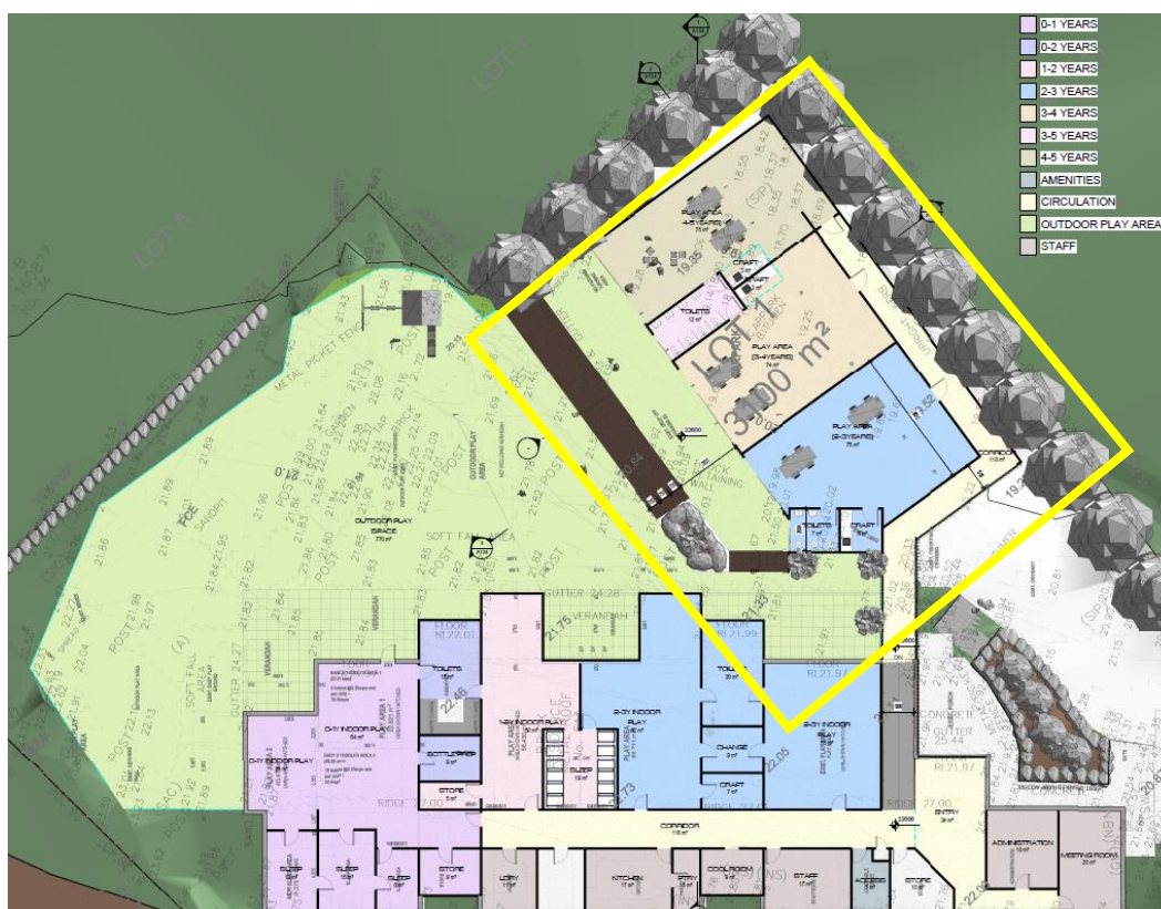
Figure 2-2: Floor plan of proposed extension (highlighted in yellow) above existing parking spaces.
