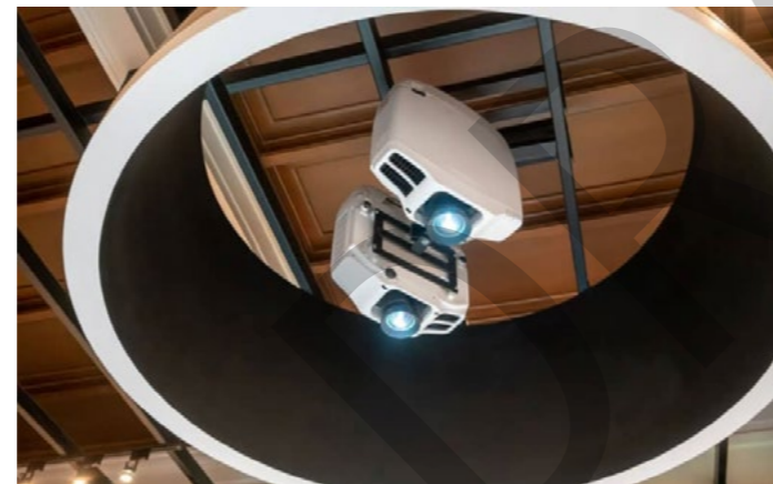
Example of ceiling-mounted vertical projection.
