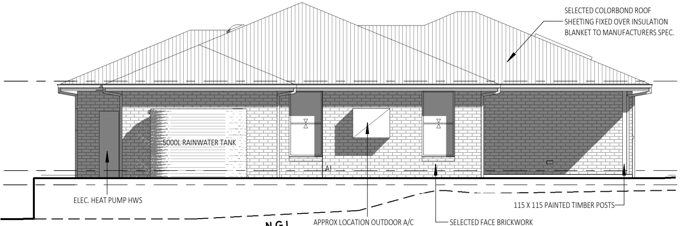
EAST ELEVATION (H2) 1 : 100
