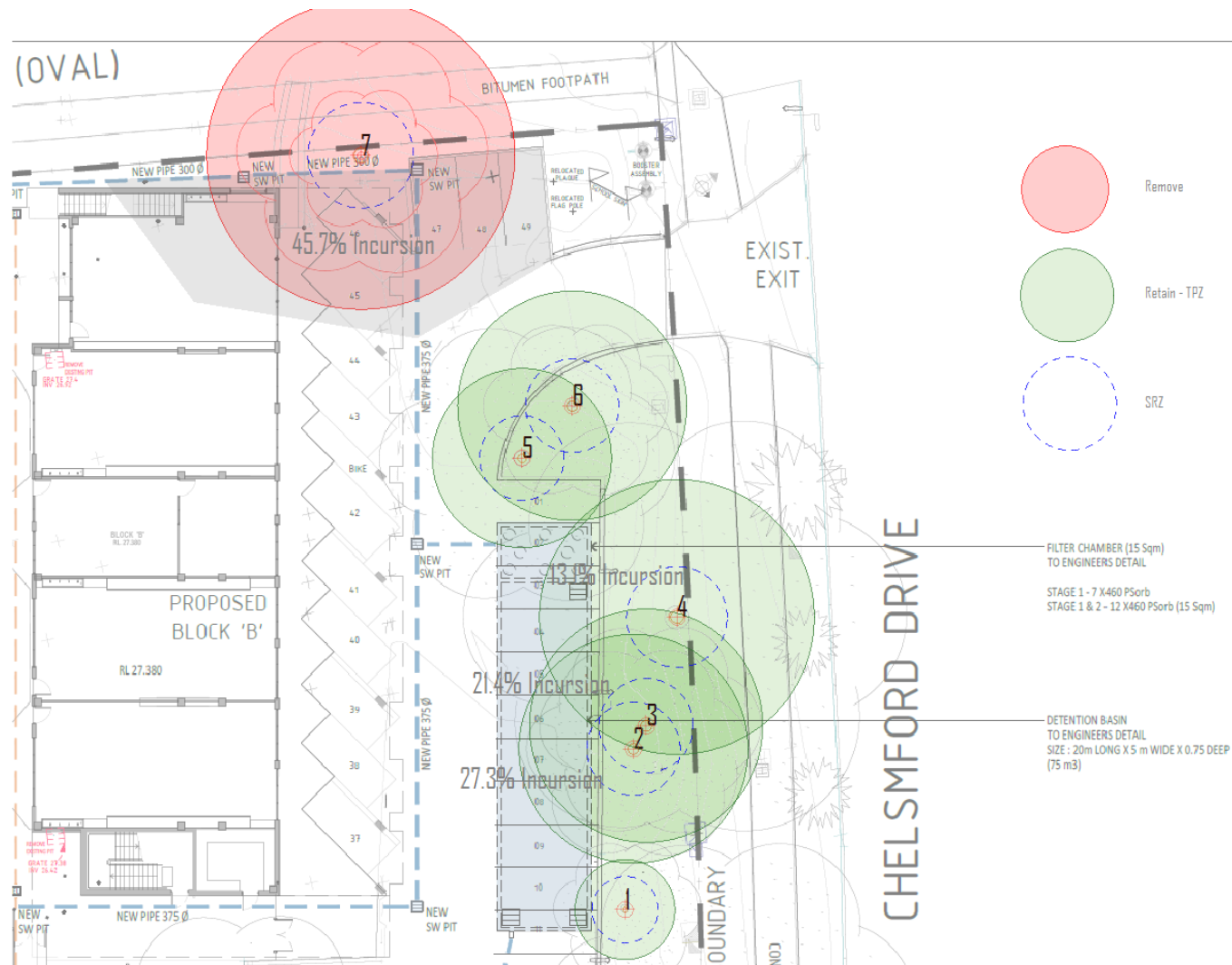
Figure 1 – Tree map showing TPZ and SRZ circles around trees and all major incursions (more 10%).
