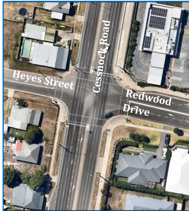
Figure 6d: Signalised intersection of Cessnock Road with Heyes Street and Redwood Drive Aerial View
