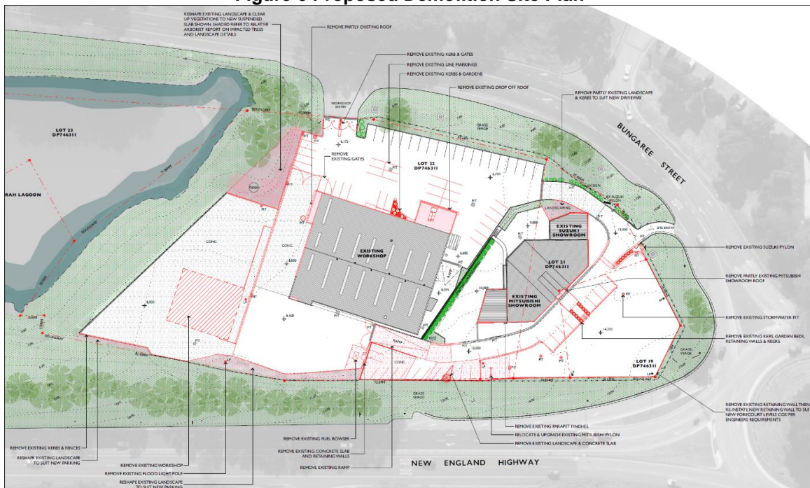
Figure 6 Proposed Demolition Site Plan
