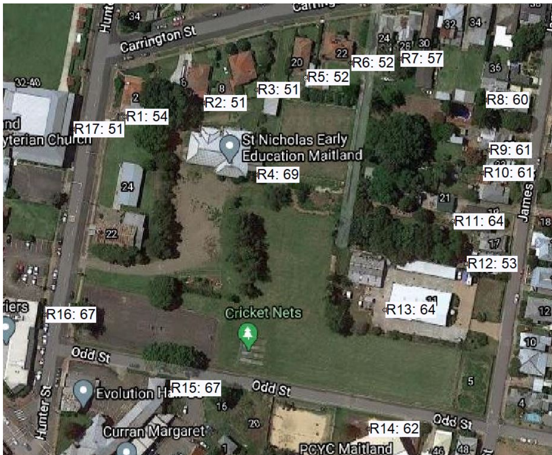
Figure 4-2 Excavation dB(A) Leq(15min)
