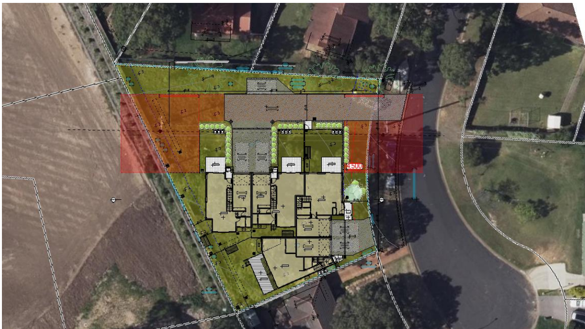
Figure 4 – Proposed development minimum front setback of 4.5m as shown in submitted architectural plans [Base Map Source: Six Maps]
