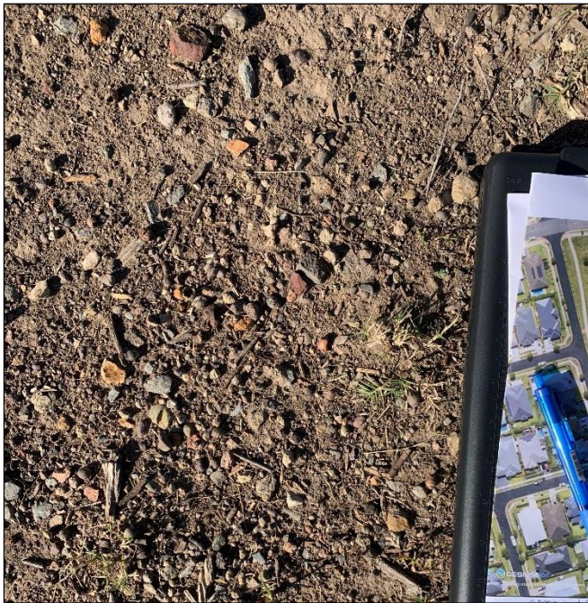
Figure 11: Exposed soil in the south-eastern and eastern portion of the site, generally comprising clayey soils and gravels.
