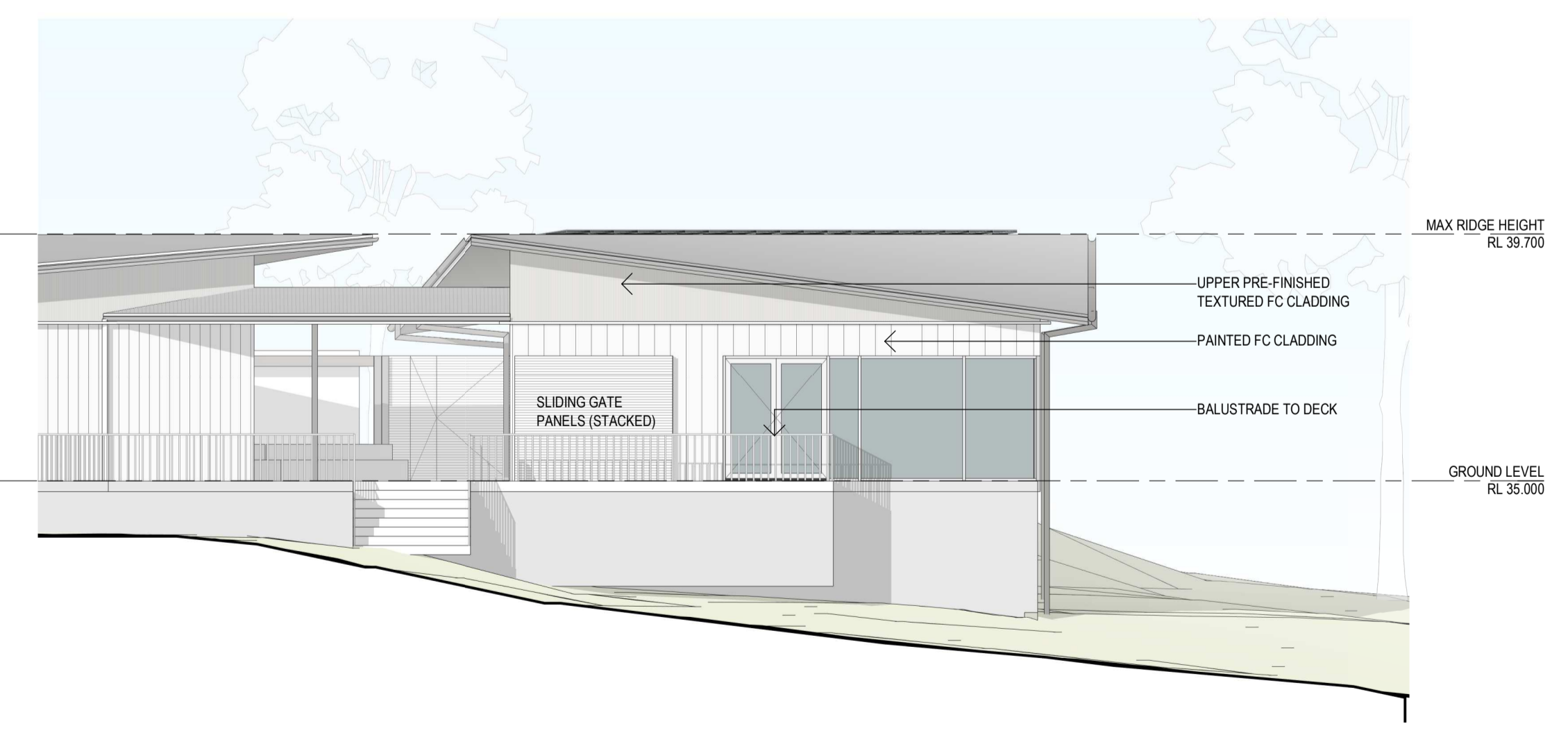
4 EAST PAVILLION - SW ELEVATION 1:100
