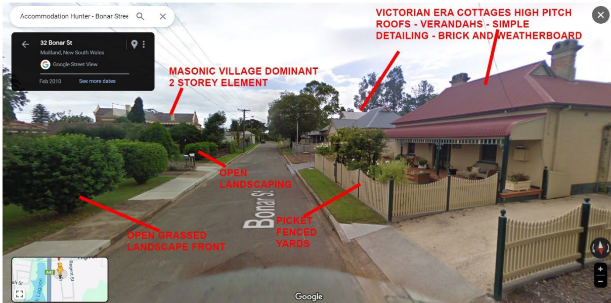
Figure 17 - View of Bonar Street Looking south. This section of Bonar Street opens into smaller allotments with more tradition Victorian era cottages. Hip and gable roofs are prominent with metal cladding. Brick or weatherboard is used. Pickets fences formalize front yards. Verandahs are also quite prominent to front facades. Additional fretwork and window awnings are also displayed.
