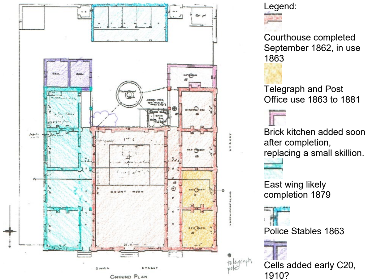
Image 27: Morpeth Courthouse, NSW - Phases of Development Source: CMP and histories, prepared by Placemark Consultants
