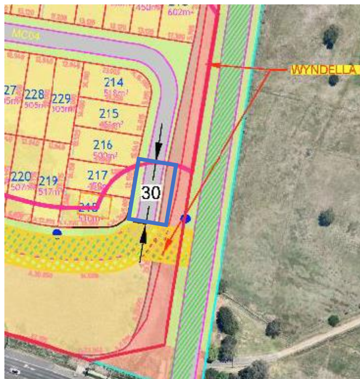
Figure 2: Proposed Parking Restricted Areas on Road MC04, based on Figure 10 of Updated BAR
