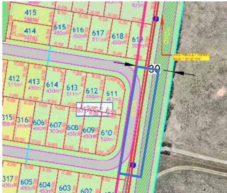
Figure 3: Proposed Parking Restricted Areas on Road MC09, based on Figure 10 of Updated BAR
