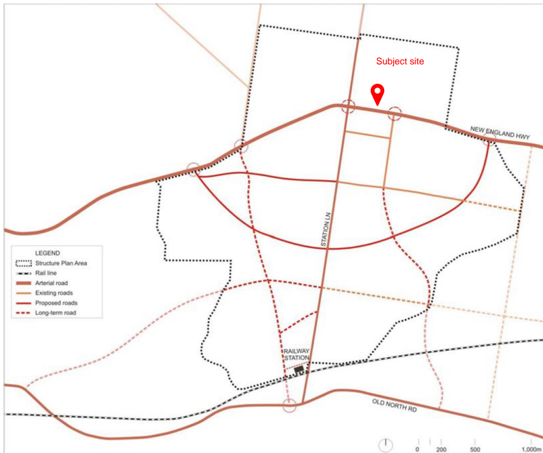
Figure 2-7 Lochinvar Structure Plan road network
