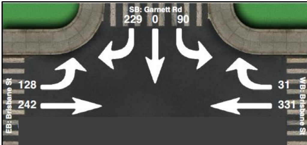
Figure 5 PM Peak (4.15-5.15pm) Traffic surveys at Garnett Road and Brisbane Street
