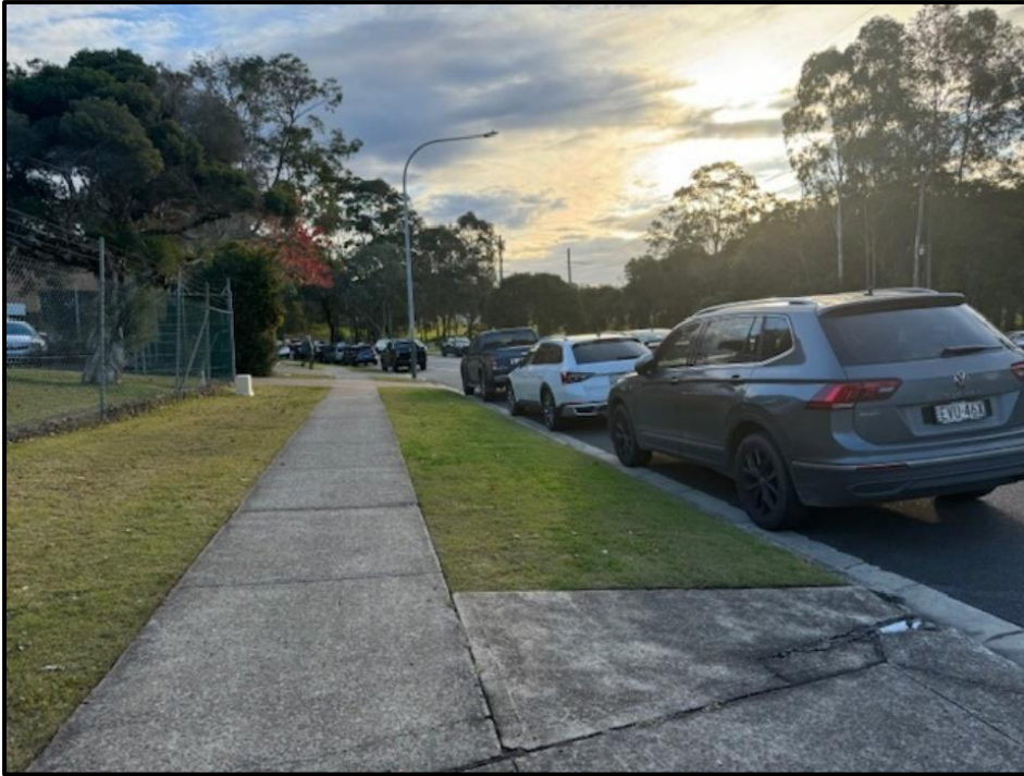
Photo 2 Sight visibility to the left (west) from the western driveway assisted by driveways but impacted by parked cars.(subject to design changes)
