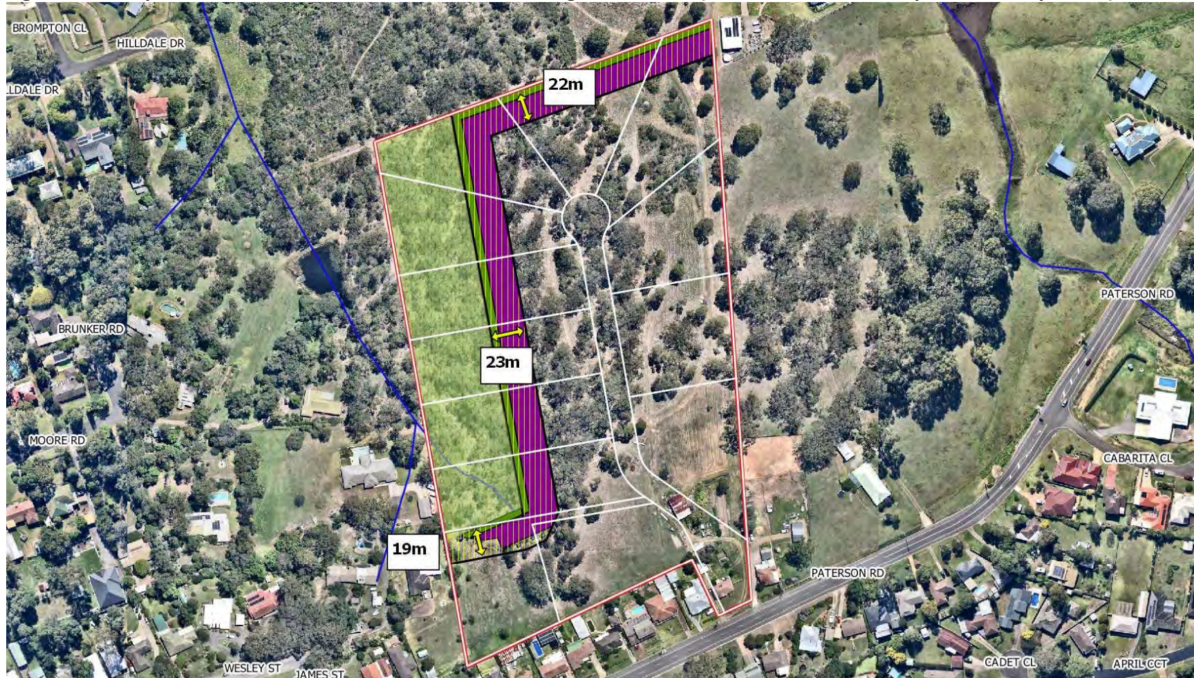
Figure 10b: Proposed Asset Protection Zone IPA & OPA management zones (from PLM Bush Fire Report dated Sept 2024)
