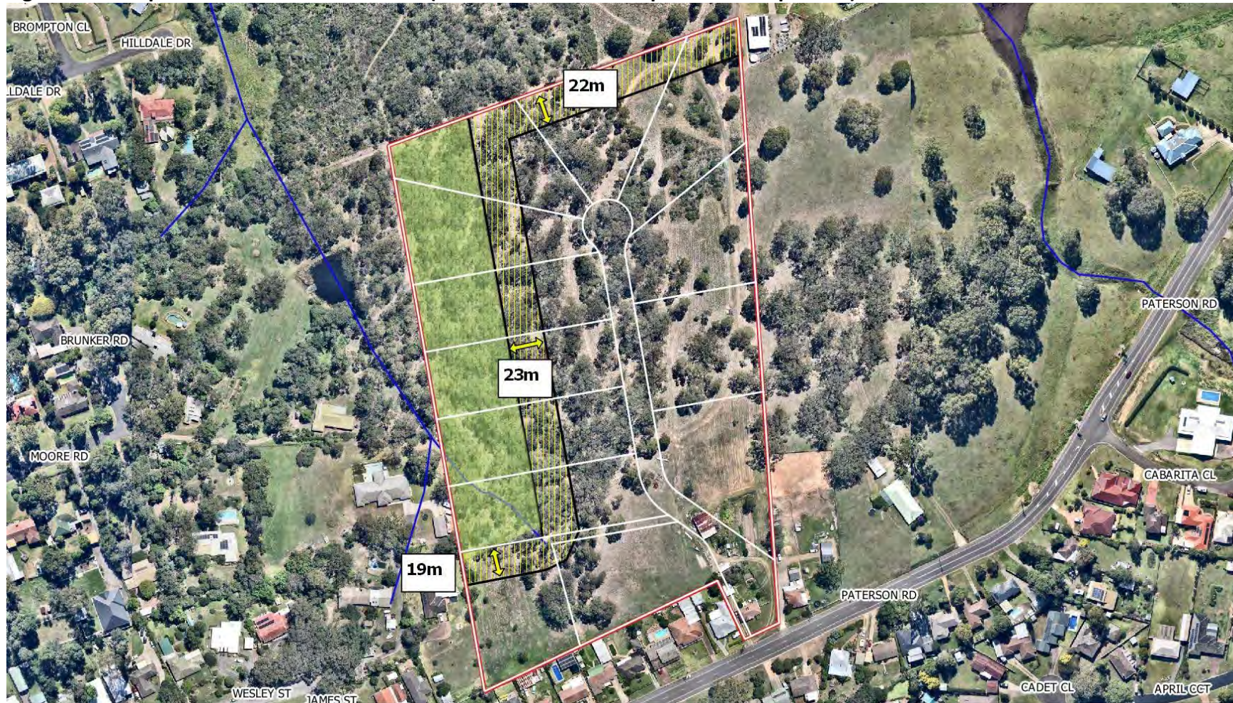
Figure 10a: Proposed Asset Protection Zone (from PLM Bush Fire Report dated Sept 2024)
