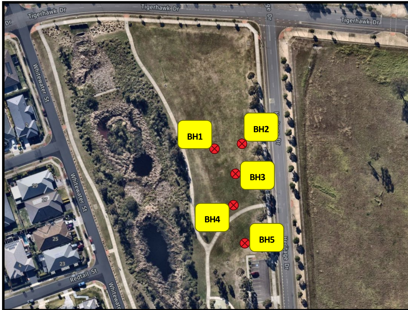
Figure 1 – Overhead image at Heritage Drive, Chisholm (Whitewater Park) showing the approximate location of the Geotechnical boreholes.
