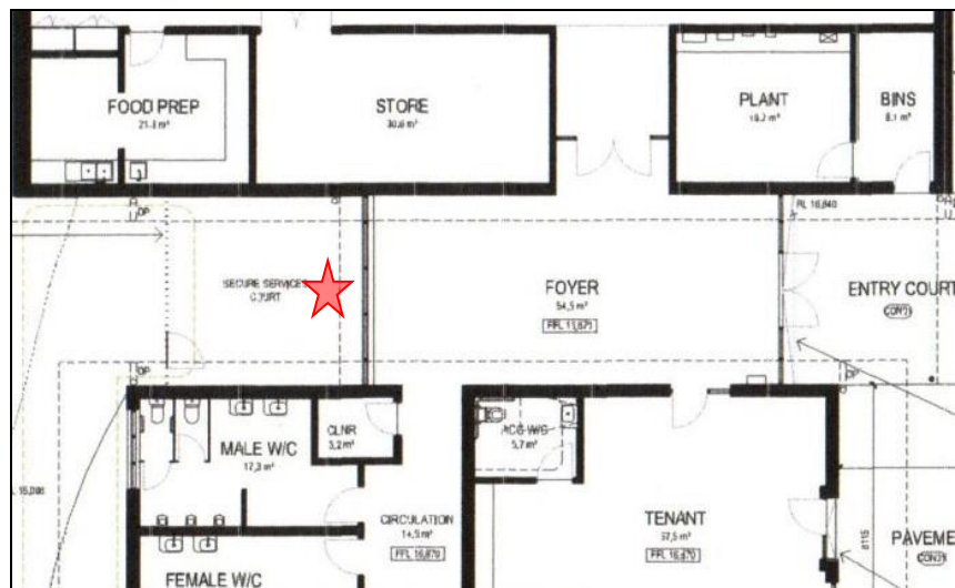
Figure 4 – A/C Condenser Location
