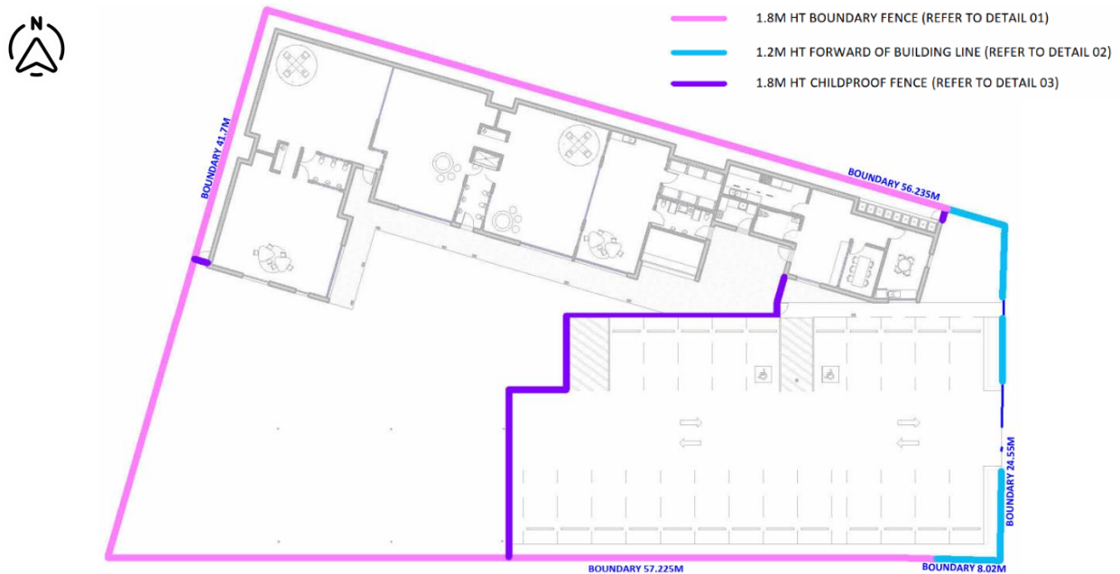
Figure 5 – Acoustic Barriers Markup (ArtMade Architects)
