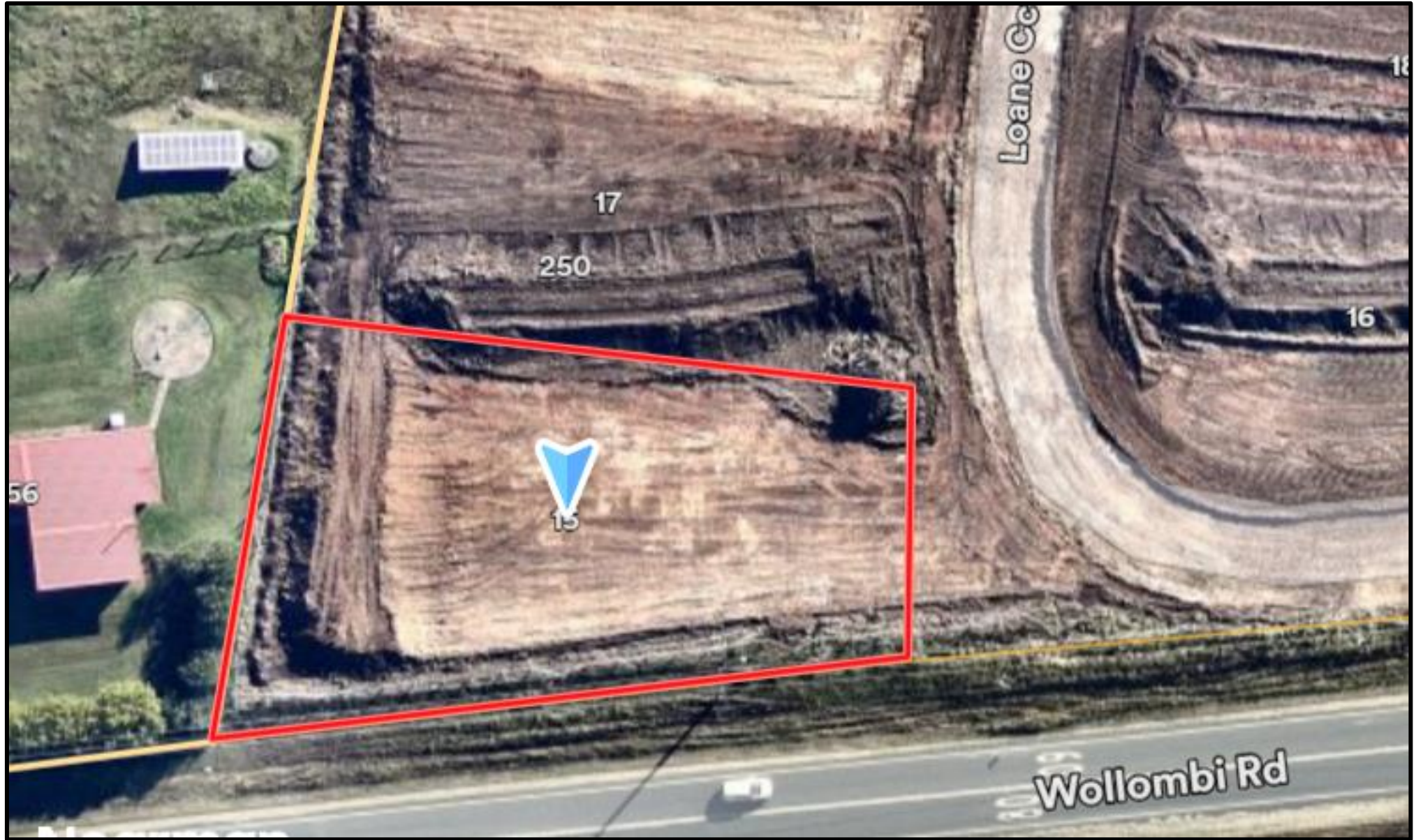
Figure 7. Aerial image of the site and surrounding area May 2023. Significant land clearing and scraping have been undertaken onsite, as well as to the property immediately north. Soil appears to have been stockpiled along the site's western boundary.
