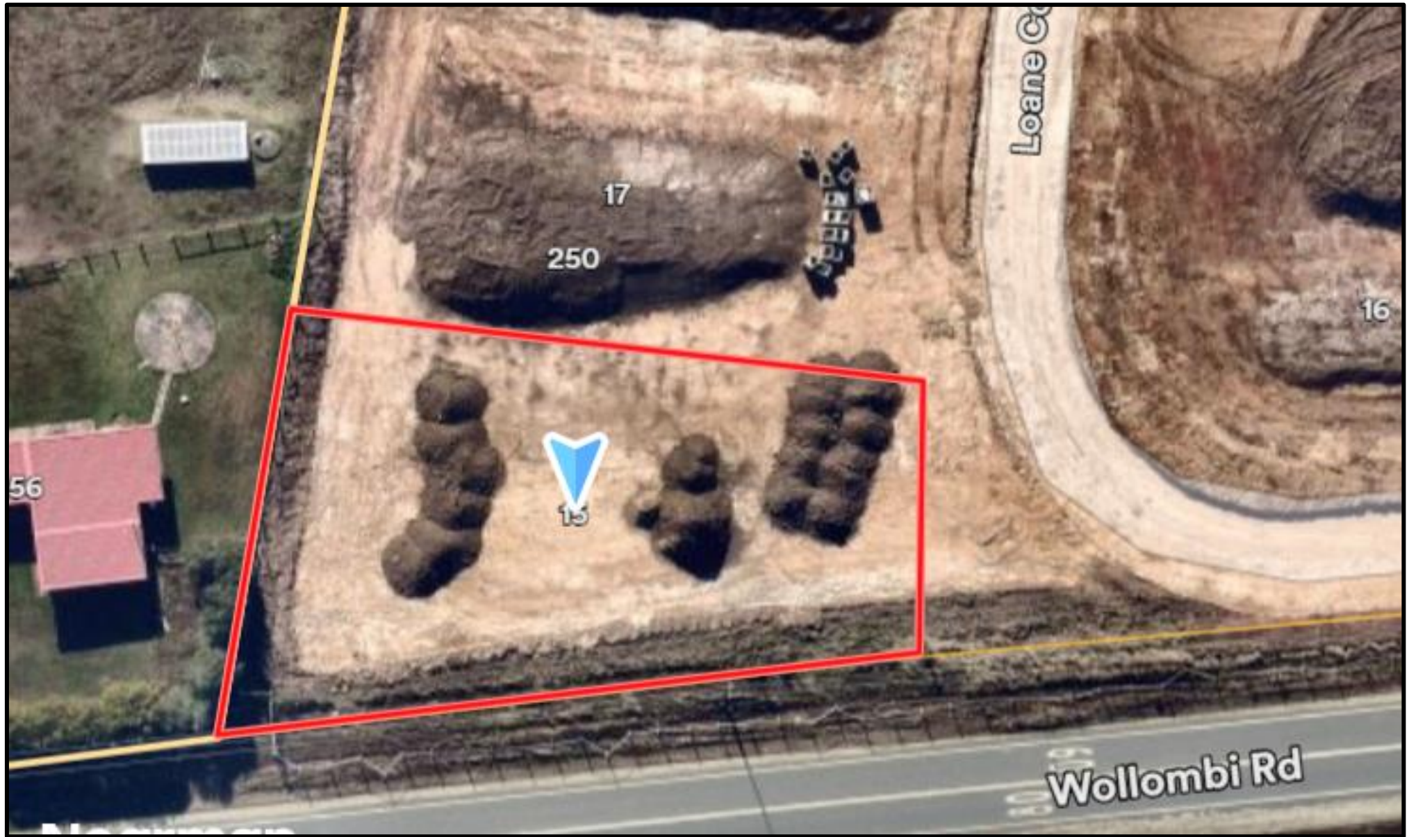
Figure 8. Aerial image of the site and surrounding area June 2023. The Site featured three large stockpiles in the center, likely imported fill material
