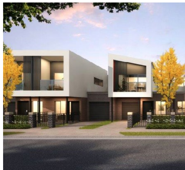
Figure 3-88 Garages are recessed elements in the streetscape
