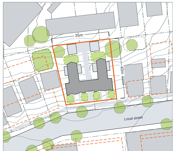
Figure 3-45 SITE SCALE: The site scale is a detailed analysis of the developments immediate context and should include the site itself, the street it addresses and surrounding properties.
