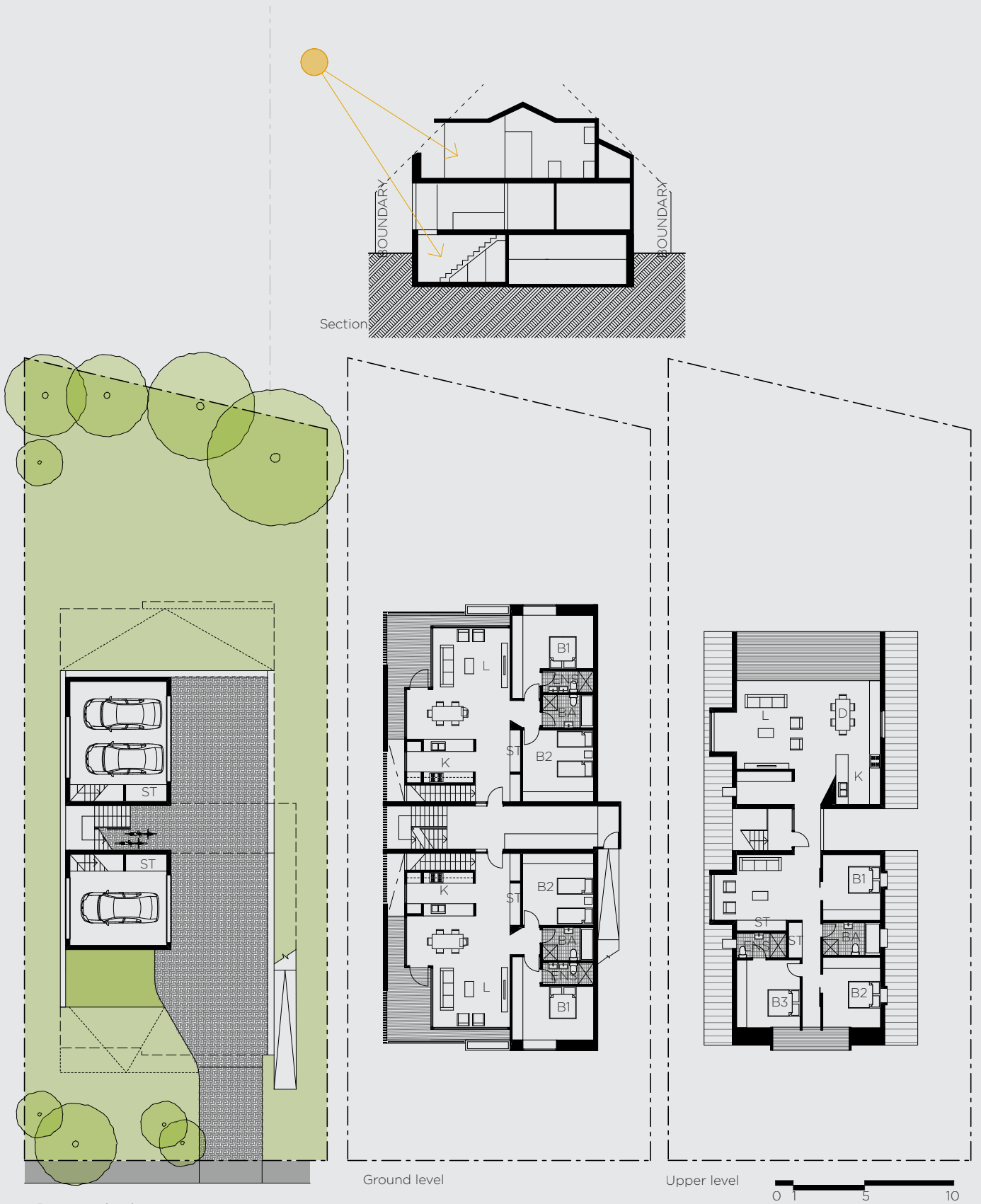
Basement level Figure 1-21 Sample plan of manor house with three dwellings and basement parking
