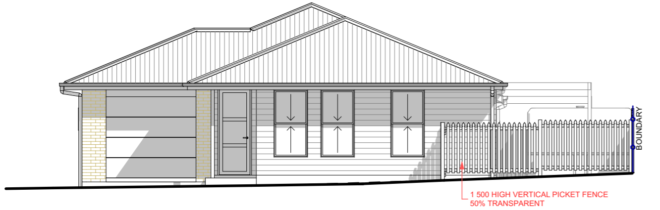
1 > RES 1 & 2 SOUTH ELEVATION 1:100
