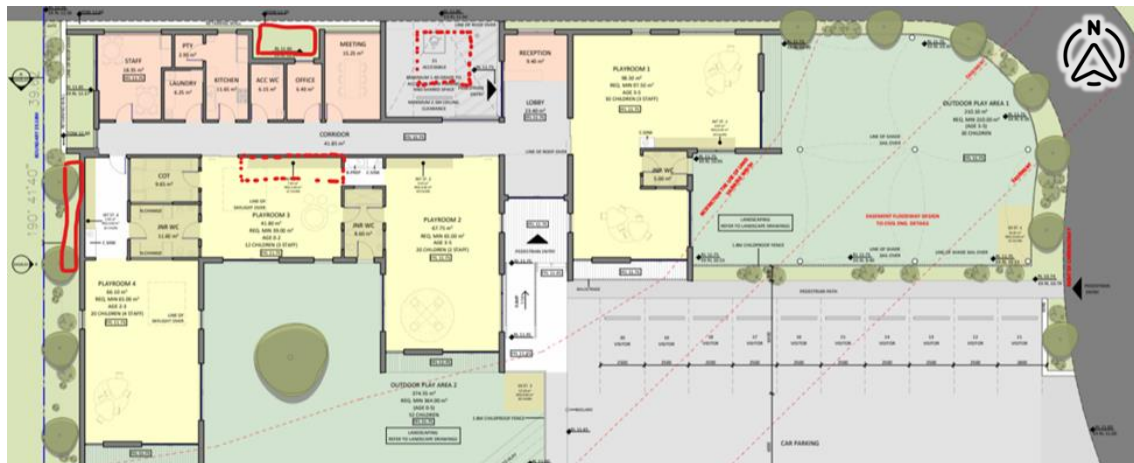
Figure 3 – Mechanical Equipment Location Markup (ArtMade Architects)
