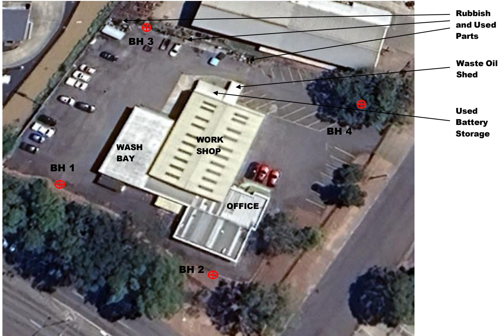
FIGURE 3 – SITE FEATURES AND BOREHOLE LOCATIONS
