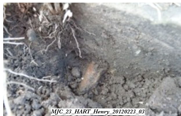
The Henry HART stele (#23, 1931) was not held securely despite cement and iron pins. At least one pin remains in the sub-base and is rusting: it will inevitably cause damage in the form of star-cracking and, subsequently, the fracturing of the stone.
