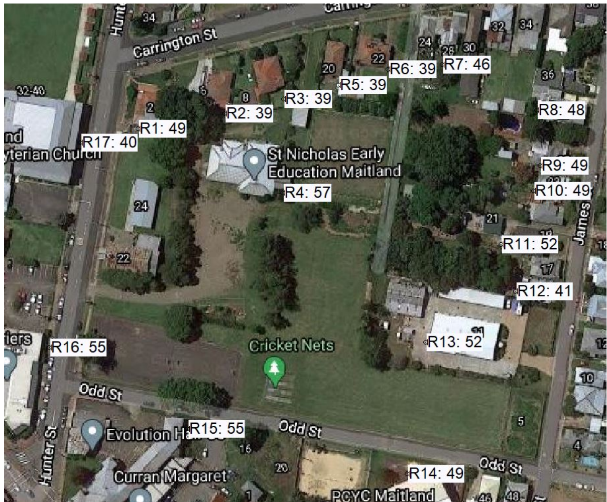
Figure 4-3 Building Construction dB(A) Leq(15min)
