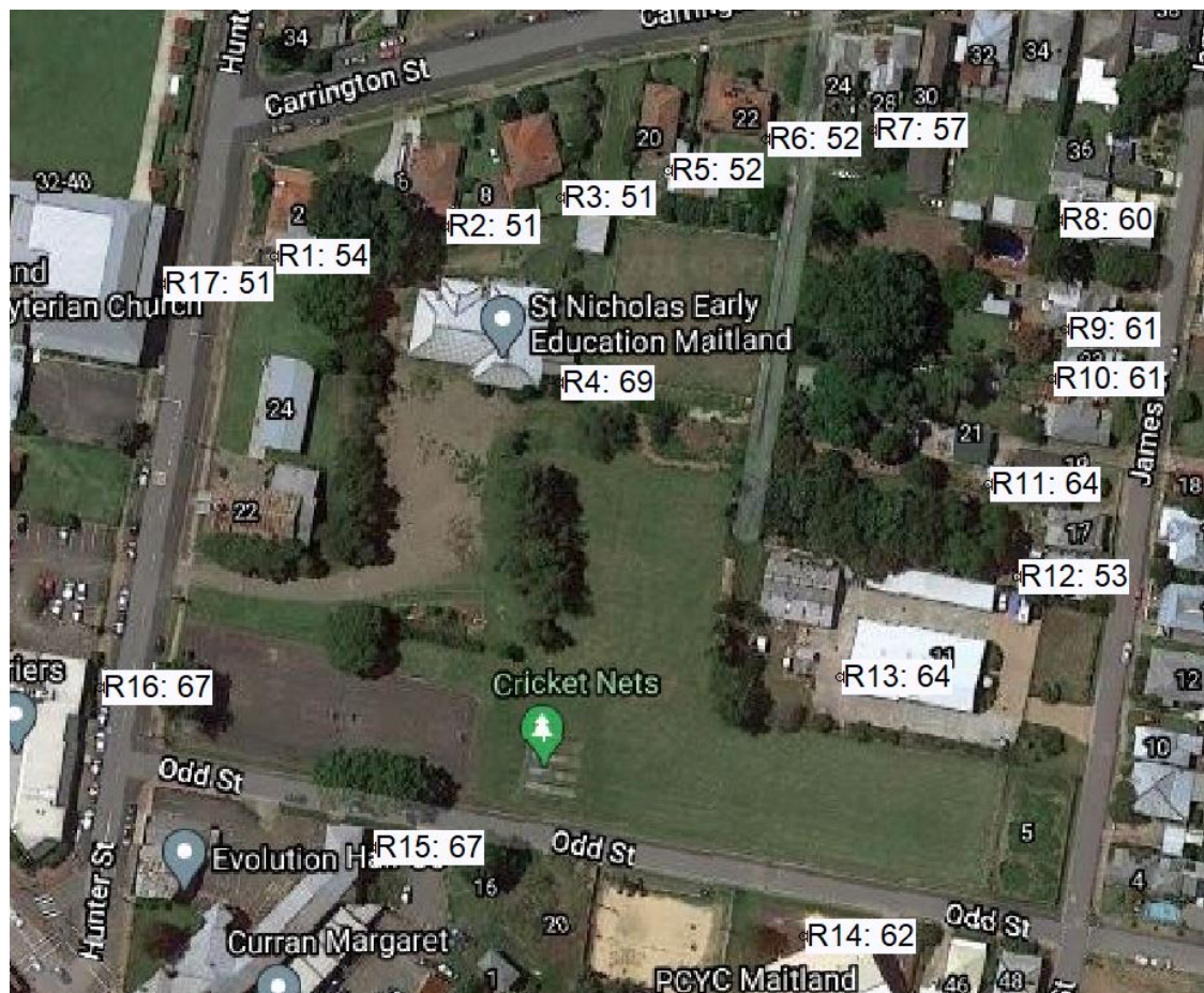
Figure 4-2 Excavation dB(A) Leq(15min)
