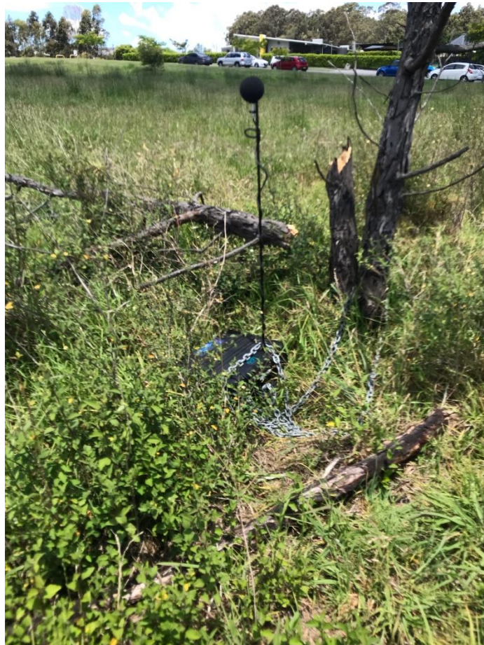
Figure 3 – Photograph of noise monitor installed on site
