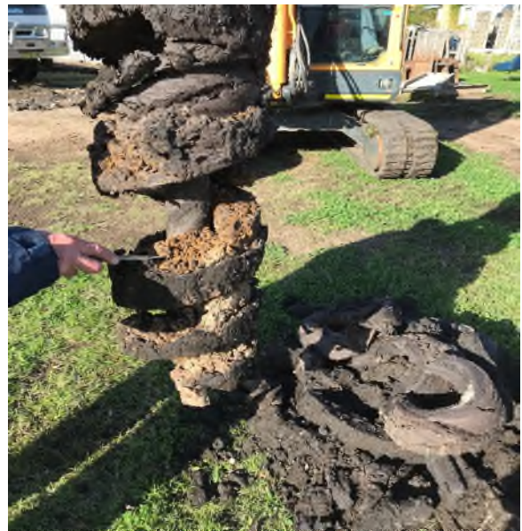
Photograph 24: Showing residual clays and sandy clays observed in BH13
