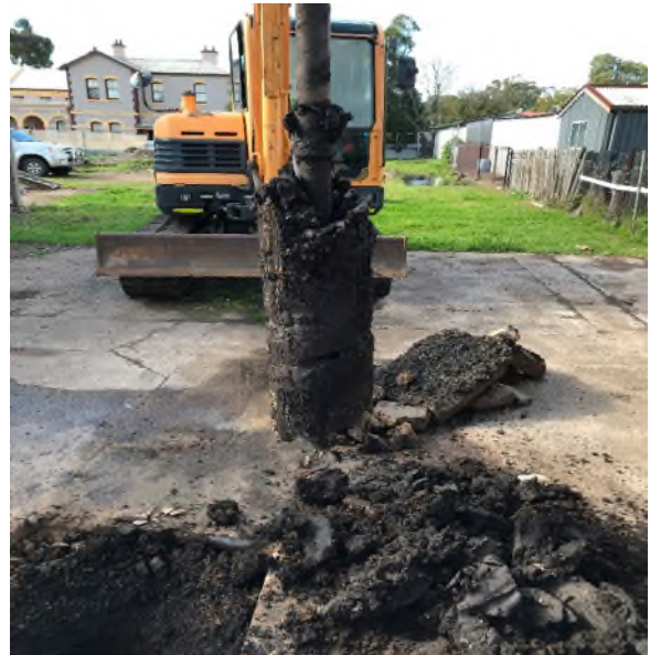
Photograph 22: Showing soil profile of BH01, sandy clays
