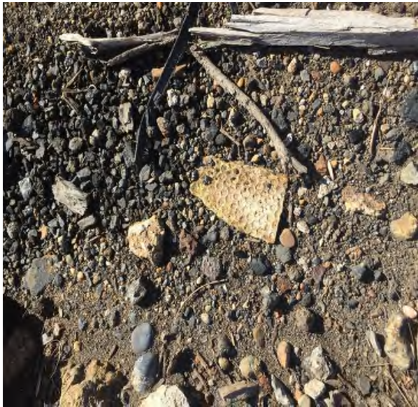
Photograph 11: Showing fragment of ACM at southern base of stockpile
