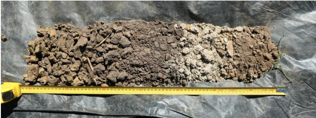
Figure 5 – Typical Soil Profile to a depth of 700mm. (Photo: Arterra 15/4/2020)
