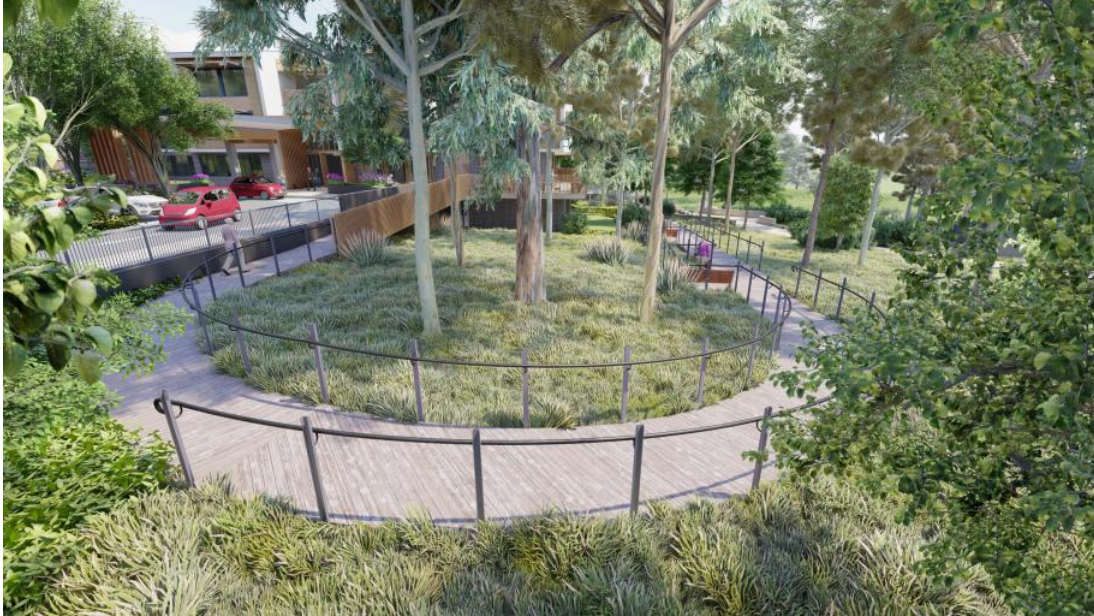
Figure 11 – Area adjacent to important trees T222-229 illustrating the low impact construction of a pedestrian boardwalk that will float just above the existing ground levels and be supported by screw piles. No grading or services are proposed in the TPA. All boardwalk work is contained outside of the SRZ of the trees. (Image Source: Arterra accurate site model render)
