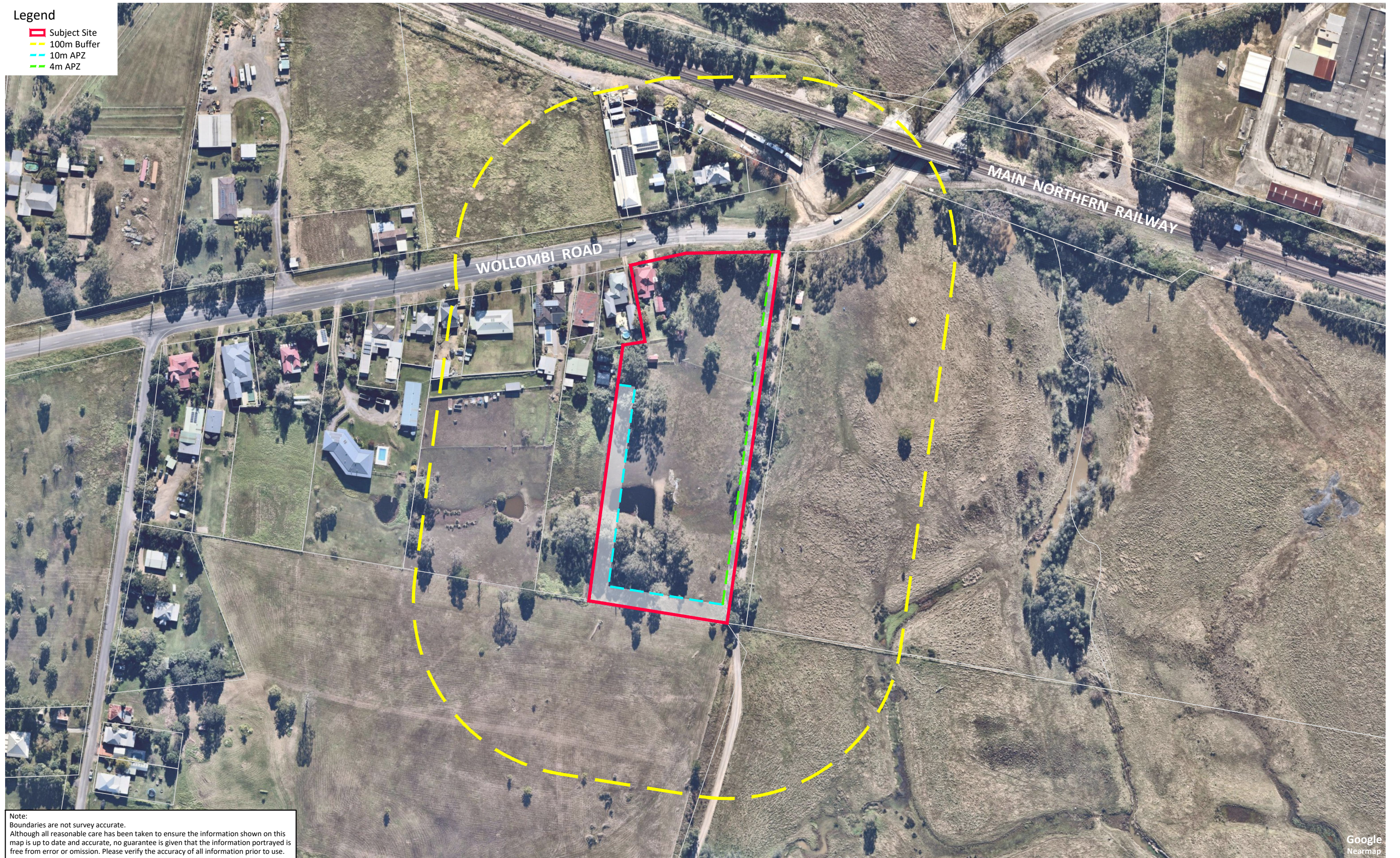
FIGURE 5-1: ASSET PROTECTION ZONES
