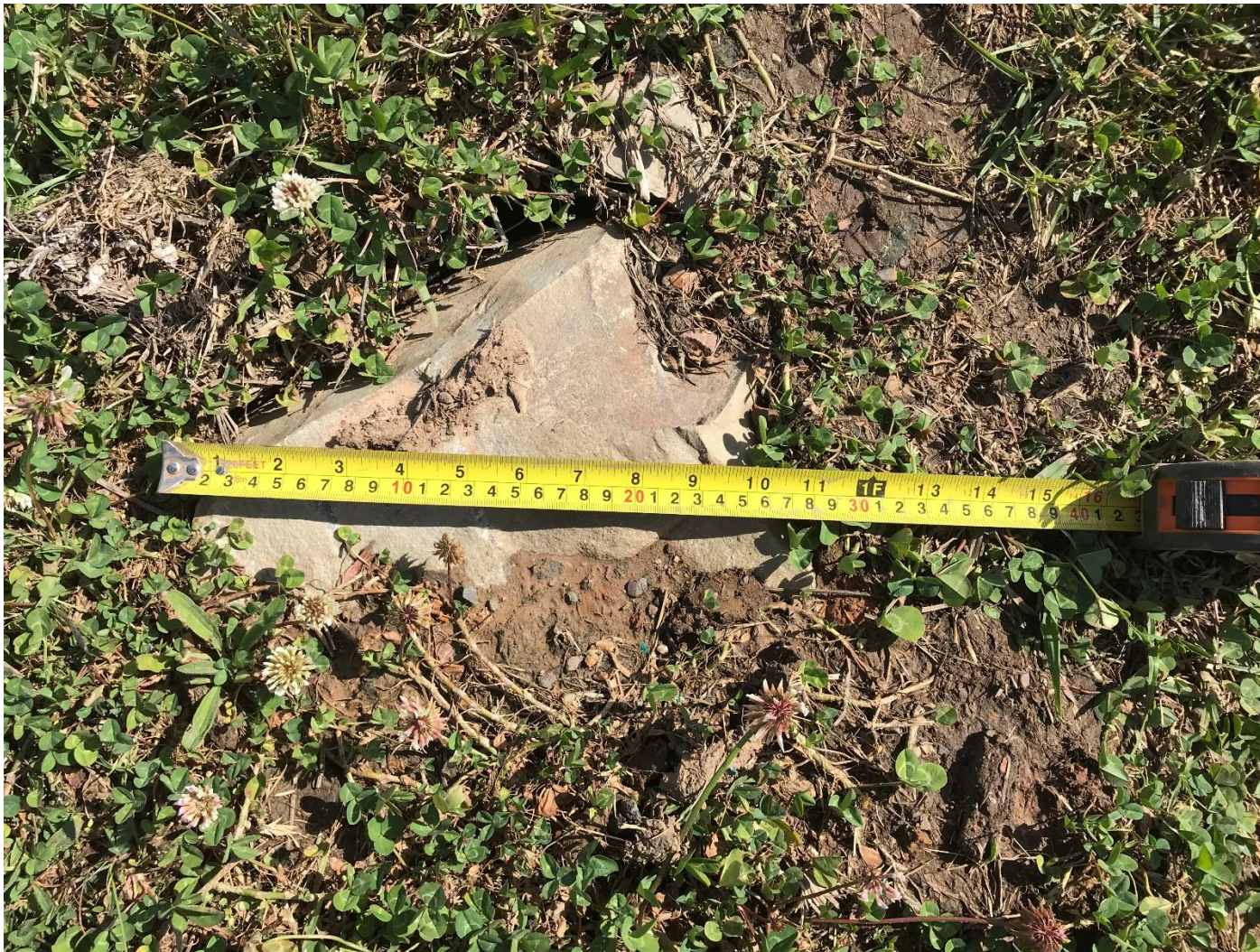
Photograph 6 – Looking example of oversize observed in fill material at the site
