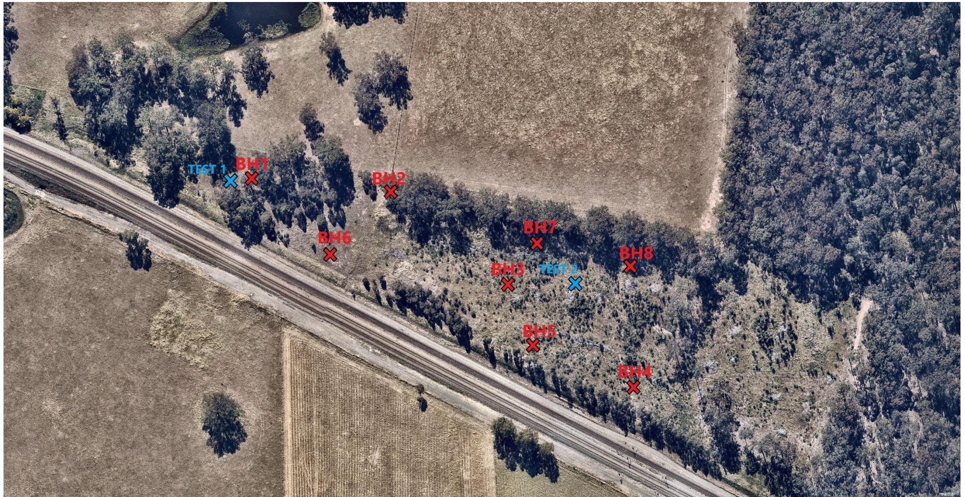
Figure 1 – Plan of the development at Lot 19 No.91 Gardiner Street, Rutherford showing the approximate location of the Geotechnical boreholes.
