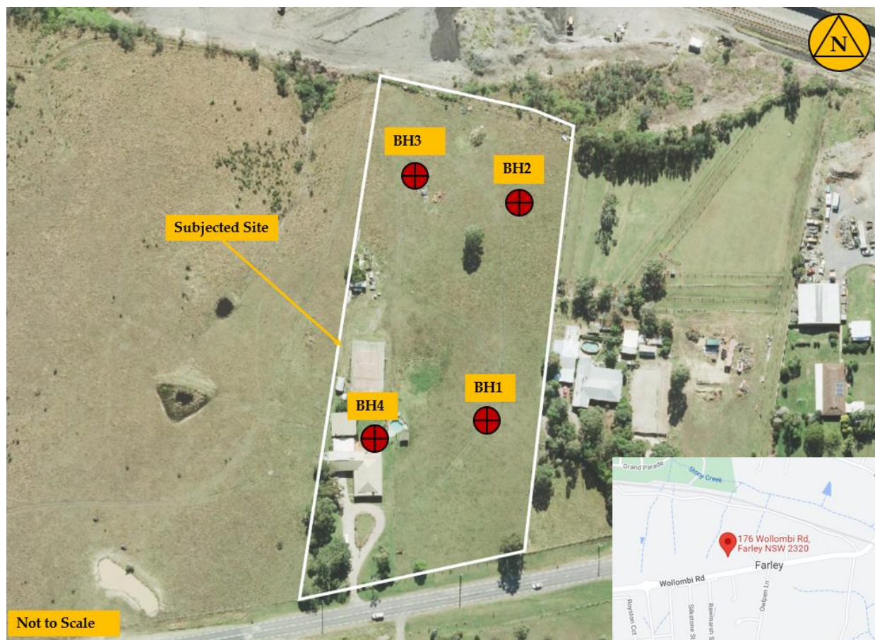
Figure 1: Site Plan and Boreholes
