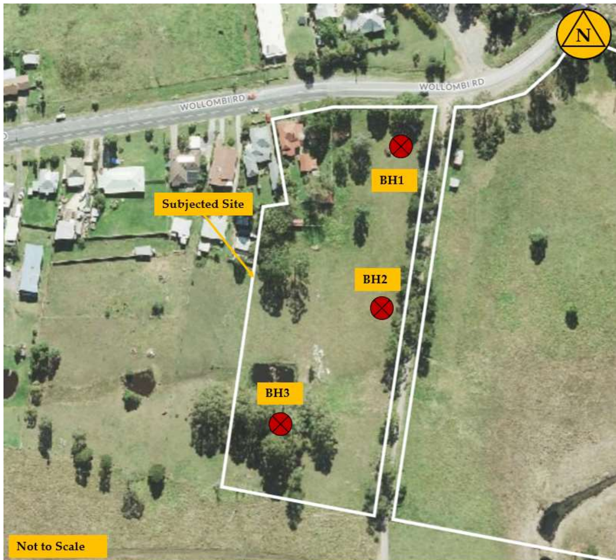
Figure 1: Site Plan and Boreholes
