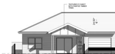
Figure 29. Unit 10 east elevation facing the entry driveway. Source BDD
