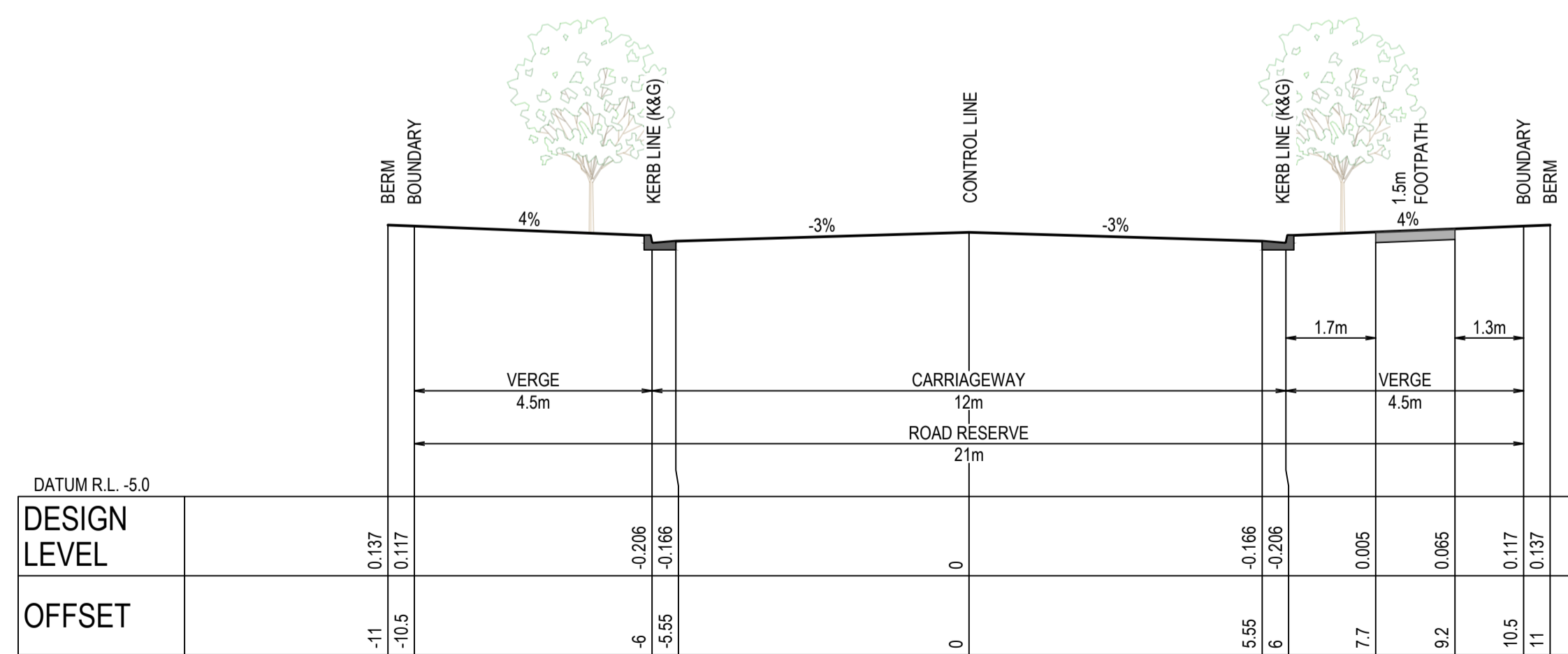
ROAD TYPE 3 - PRIMARY COLLECTOR (12m WIDE PER LOCHINVAR U.R.A. DCP) SCALE 1:100 NATURAL
