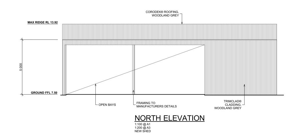
CORODEK® ROOFING, WOODLAND GREY MAX RIDGE RL 13.92 GROUND FFL 7.50 TRIMCLAD® CLADDING, STEEL FRAMING TO
