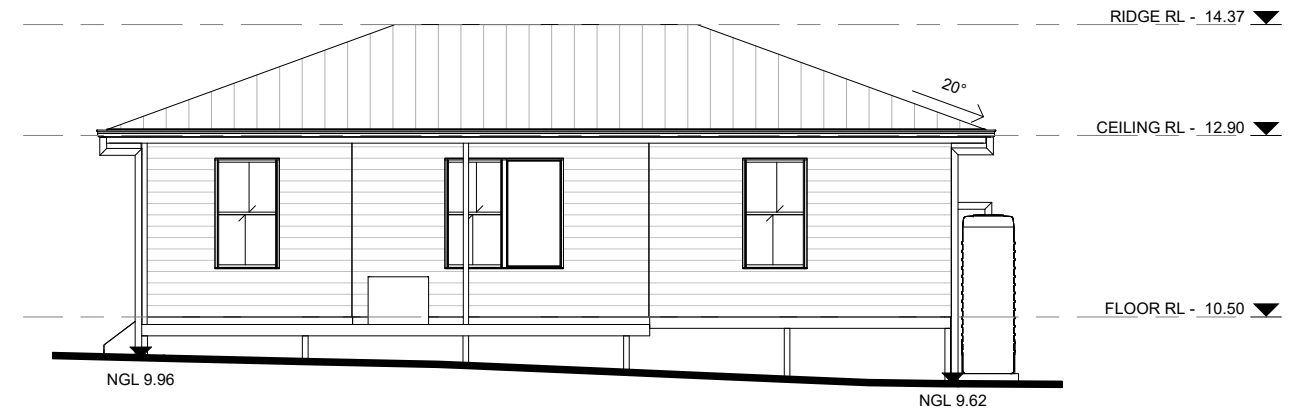
4 SOUTH WEST ELEVATION 1 : 100
