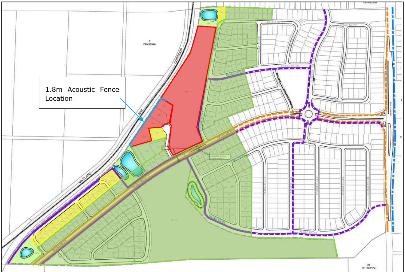
Figure 4-1: Zones for minimum architectural upgrades for a freight train travelling at maximum 30km/hr
