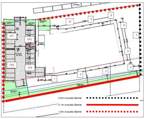
Figure 5 – Proposed Acoustic Fencing Plan
