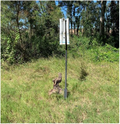
Photograph 3: Dust Deposition Gauge 13 April 2021
