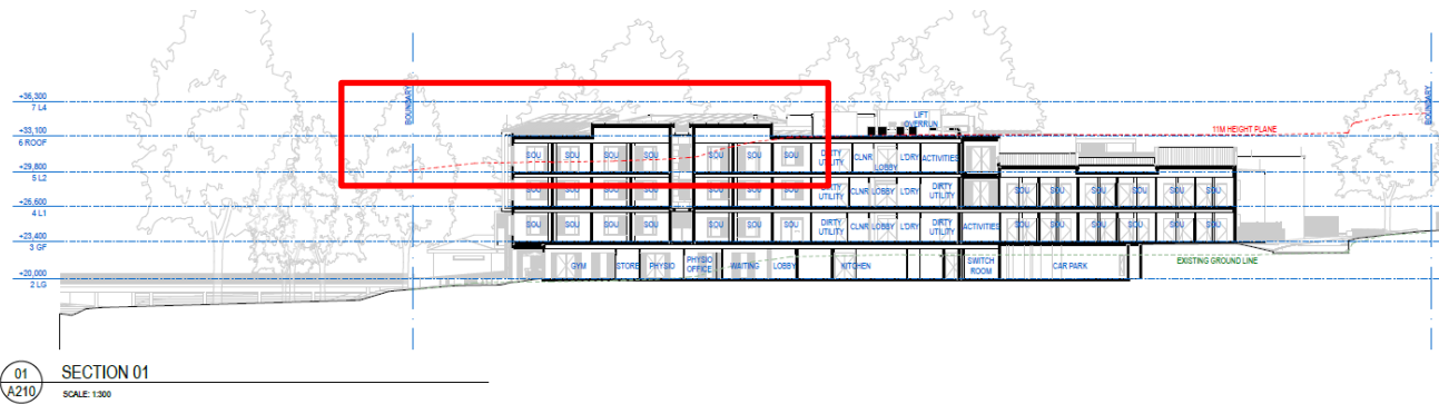
Figure 24 Section illustrating where the topmost habitable ceiling exceeds the 11m DCP height limit (dotted red) Source: Calder Flower Architecture
