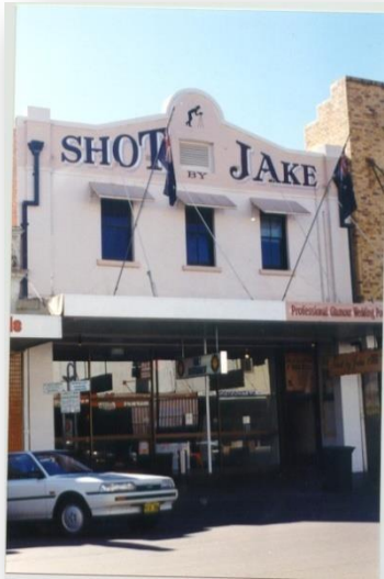
Signage should be located within architectural elements of the building using appropriate lettering style, size and colouring.
