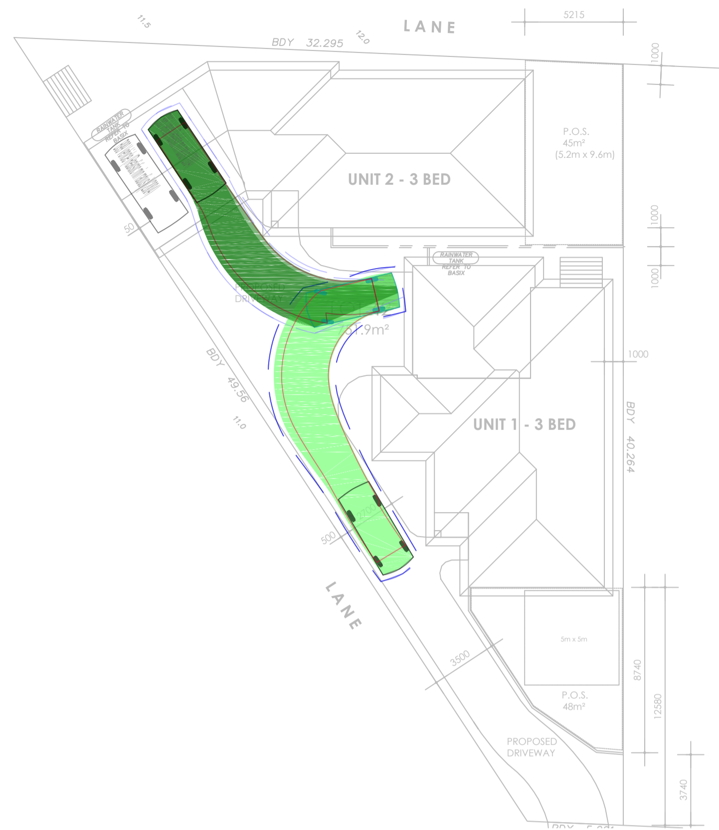
B85 UNIT 2 GARAGE EXIT TURNING PATH 1:200
