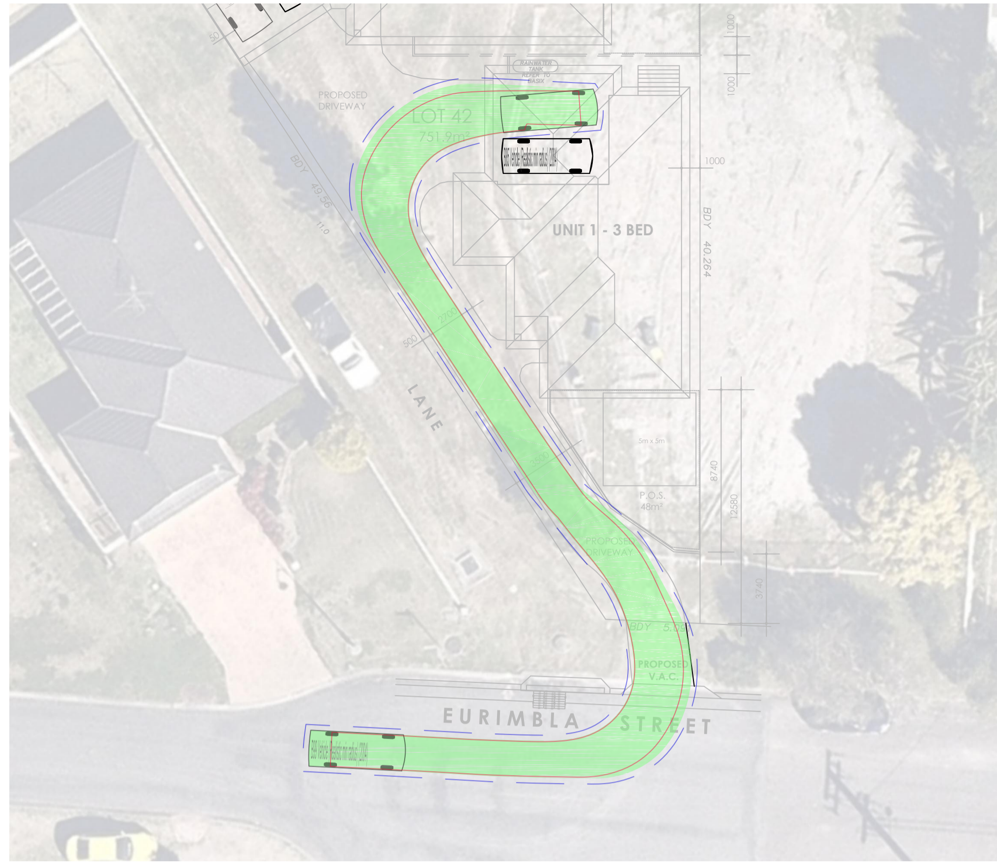
B99 SITE INGRESS TURNING PATH 1:200
